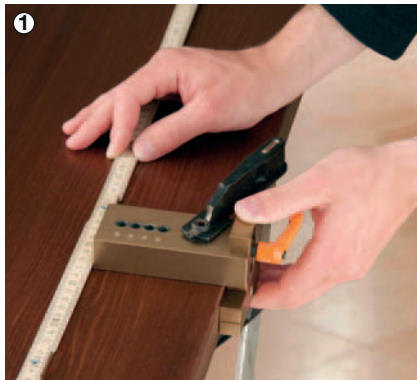
1 Place HCS® jig at required handle height on door and tighten.
